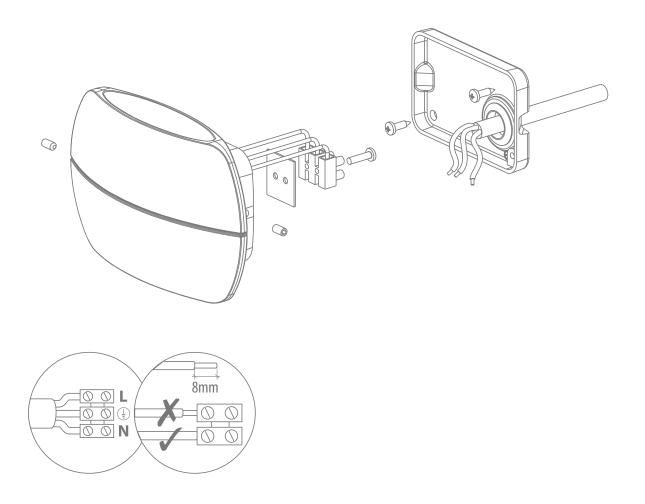
**Note:** -The lamp must be installed by professional electrician
